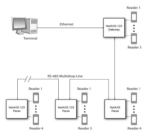
Figure 10: RS-485 Configuration via NetAXS-123 Gateway
